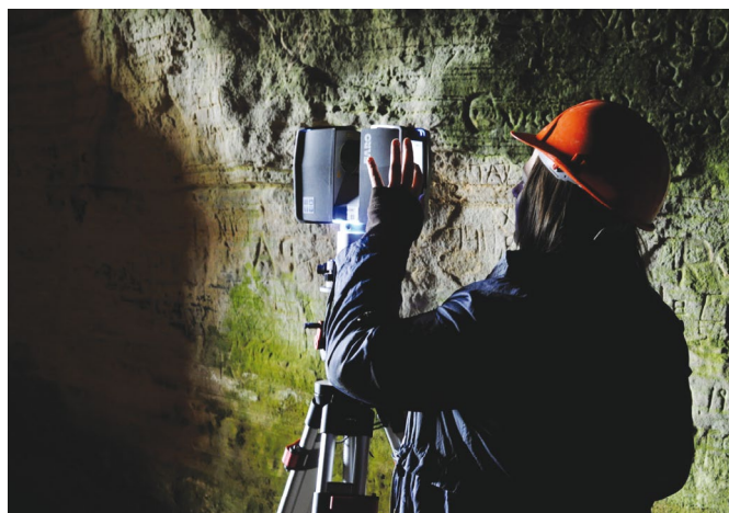
Terrestrial laser scanner in operation at the Sculptor's Cave. Photograph © The Sculptor's Cave Project
